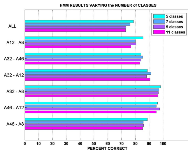
Fig. 3. (Color online) Hidden Markov model results showing the dependence on the number of states in the model. Two Gaussians and 24 cepstral coefficients were used in the calculations
