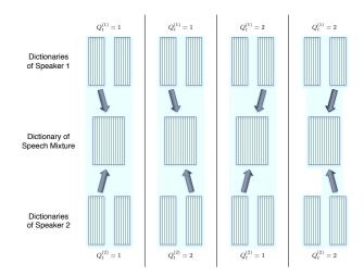
Fig. 3: Combining dictionaries of two sources to model a mixture. In this simple example, each source has two dictionaries so there are a total of four ways of combining them.
